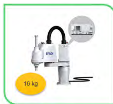
The T3 has a built-in controller
